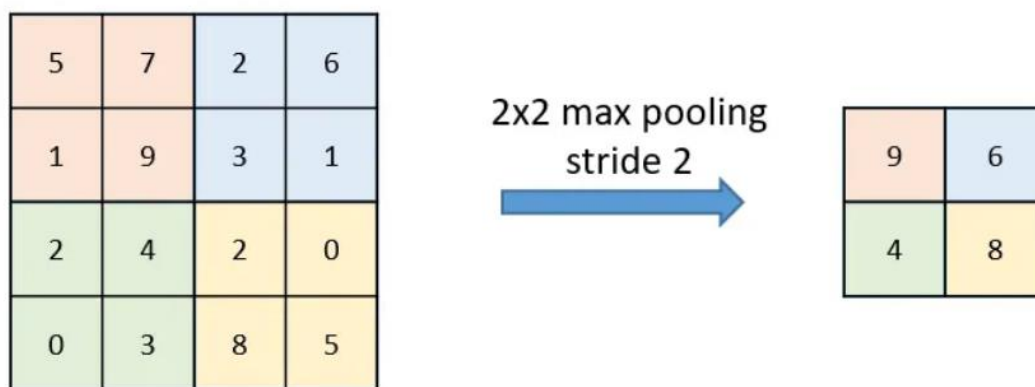
Max pooling using kernel of size 2 \times 2 with stride 2
